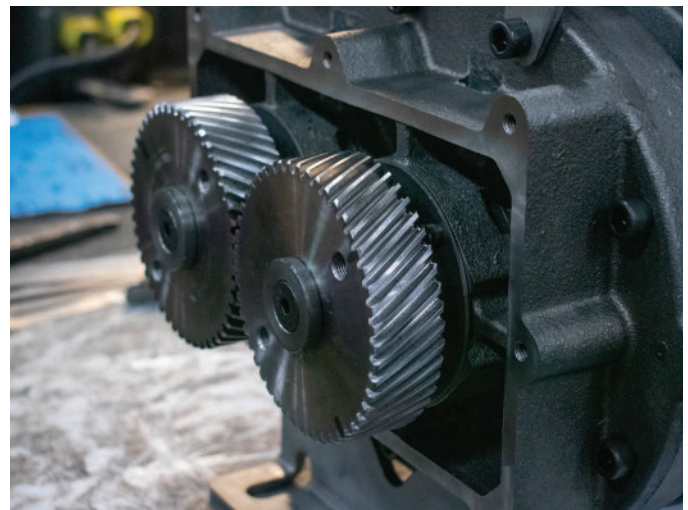
CP Series blower internal helical gears.
