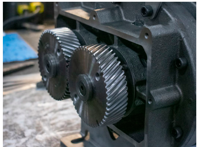
CP Series blower internal helical gears.
