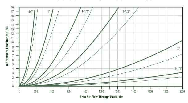
**Example #1**: A customer has a 185 cfm air compressor equipped with 100' of ¾" hose to operate a Sullair 90 pound paving breaker. The 90 pound paving breaker requires 62 cfm to operate. How much pressure loss can the customer expect at the tool if the compressor is providing 100 psig inlet pressure?
